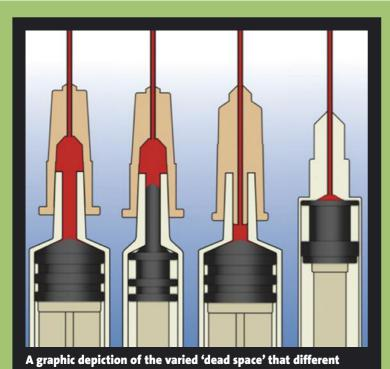
needles and syringes may contain – from left to right: a standard (high dead space) syringe with detachable needle; a low dead space syringe with standard detachable needle; a standard syringe with a low dead space needle; and a low dead space insulin syringe with a fixed needle.
